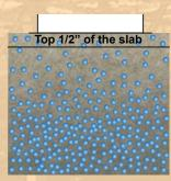
Calcium chloride is therefore only a surface test, highly affected by ambient conditions in the room or building. Even if done correctly, a calcium chloride test tells you nothing about what's going on deeper in the slab.
